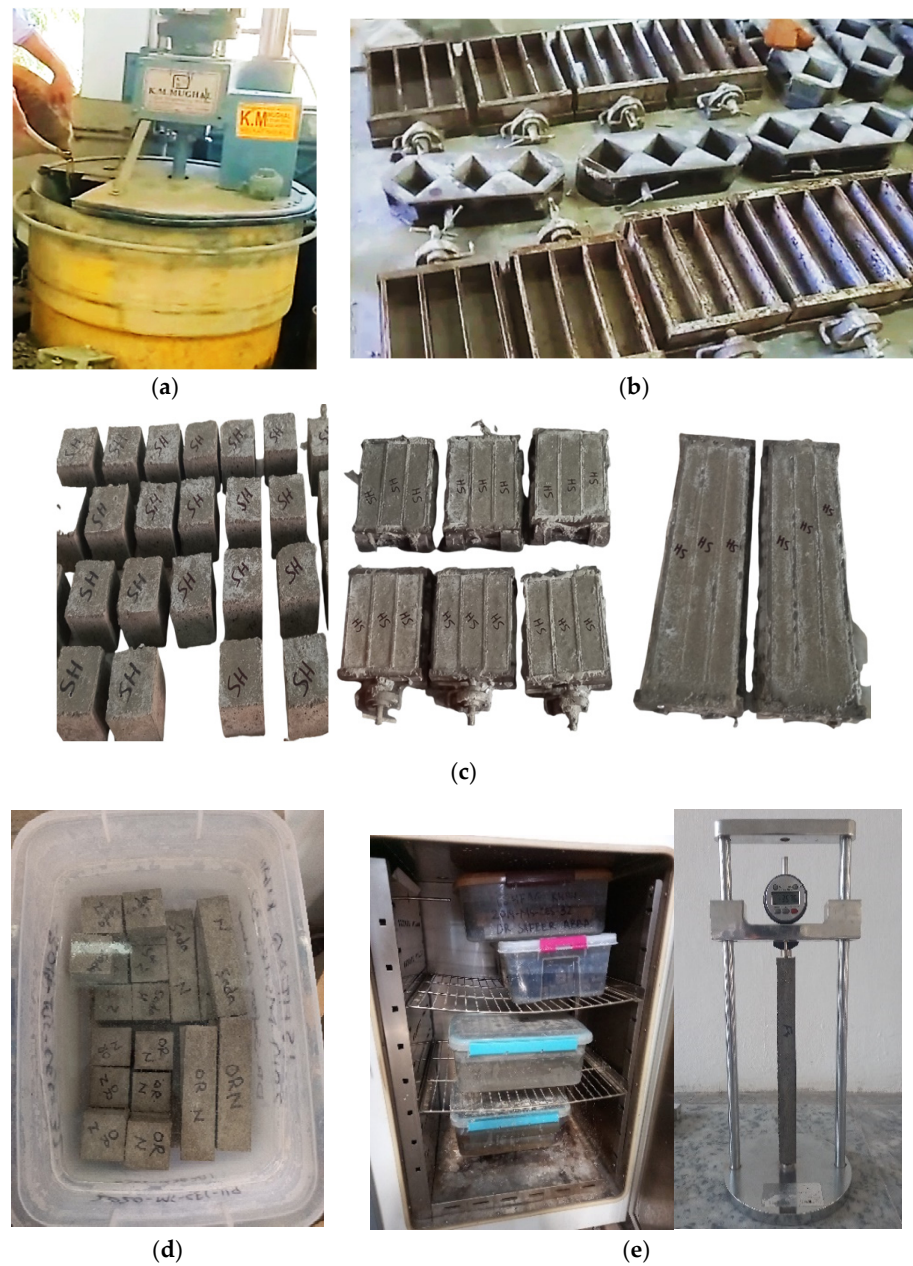
Figure 2. Specimen preparation and testing (a) Electrical mixer; (b) molds placed on vibratory table; (c) casted specimens; (d) specimens placed in ASR solution; (e) specimens placed in oven and testing using digital length comparator.
