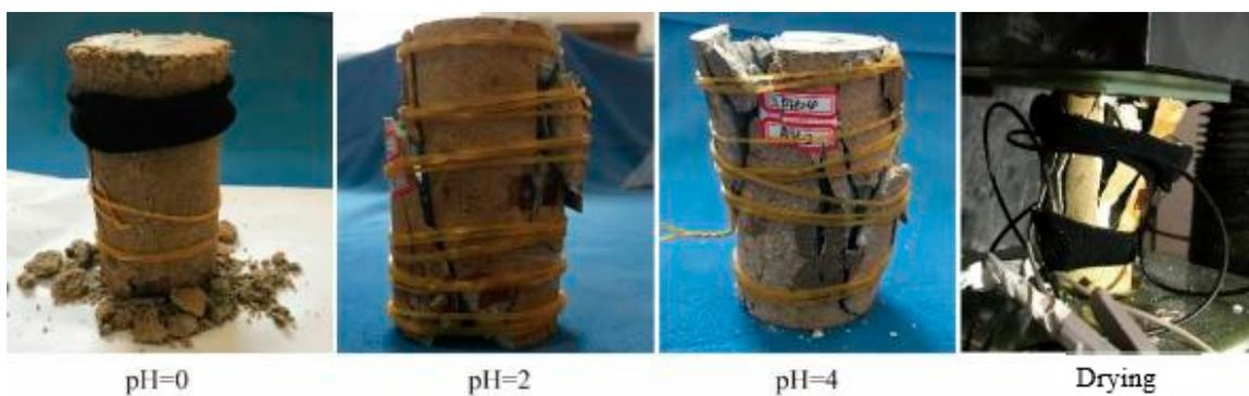
**Figure 5.** Failure features of lamprophyre.
