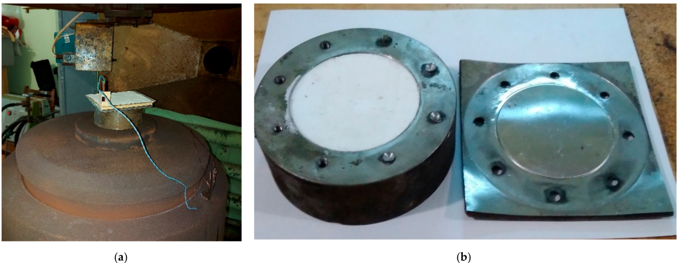
Figure 5. Powder activation by explosive loading: (a) experimental assembly mounted on the table of an explosion chamber with HE charge on top; (b) mold with treated powder after removing the steel plate.
