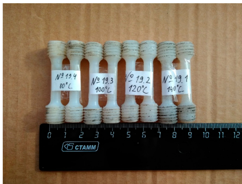
Figure 3. Tensile test samples made from compacts produced by CIC at preheating temperatures of 80, 100, 120 and 140 °C.
