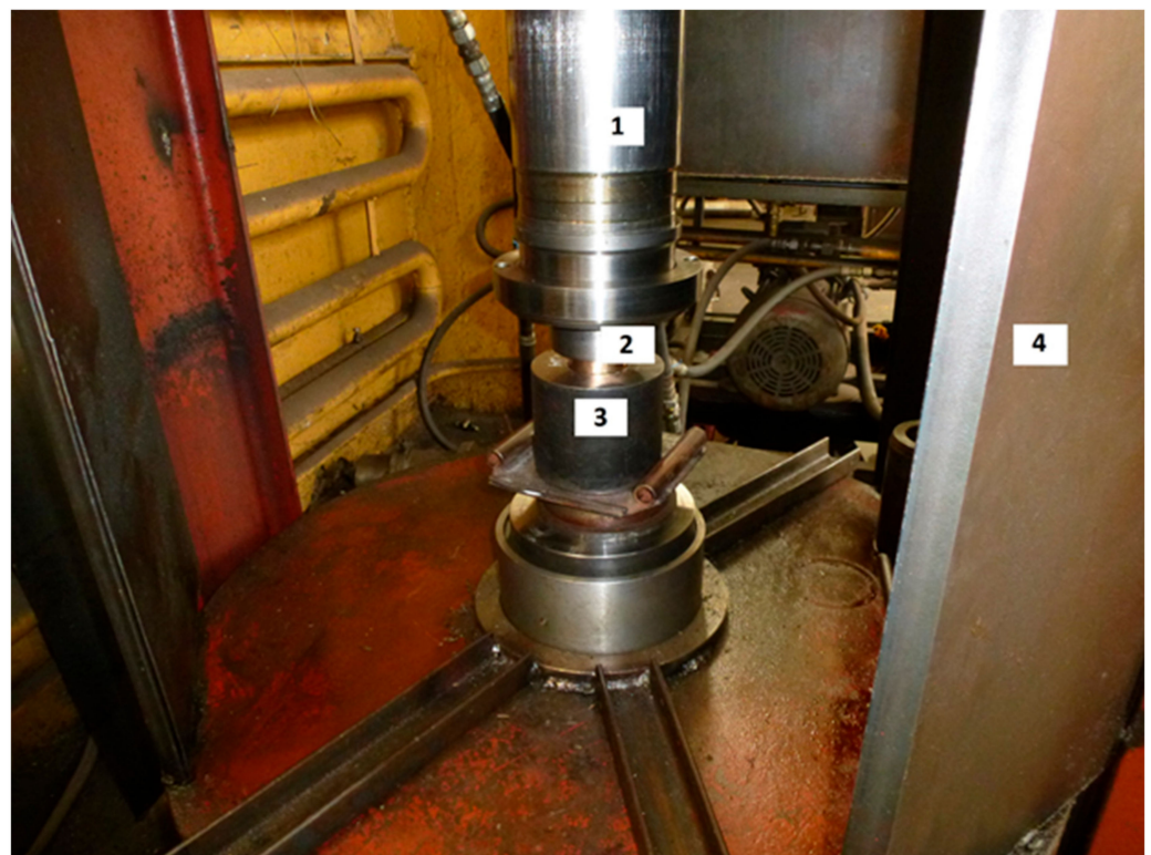
Figure 2. Hydro-pneumatic impact device for compaction of UHMWPE powder: 1, impactor; 2, piston; 3, die; 4, device housing.
