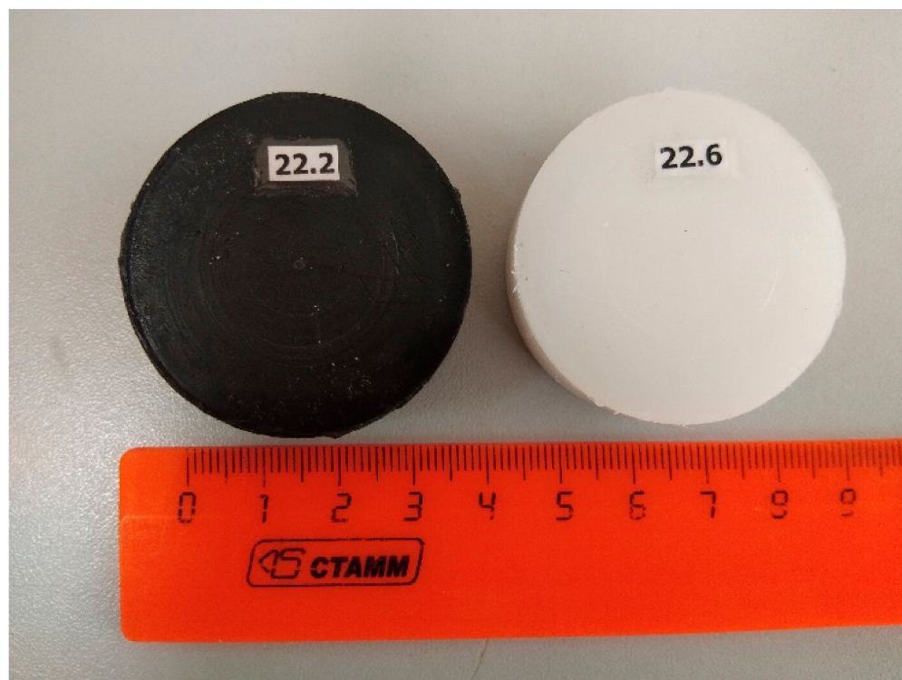
Figure 6. Compacts with a diameter of 40 mm and a height of 15 mm made of pure UHMWPE (right) and UHMWPE + 0.5 wt.% NDC (left).
