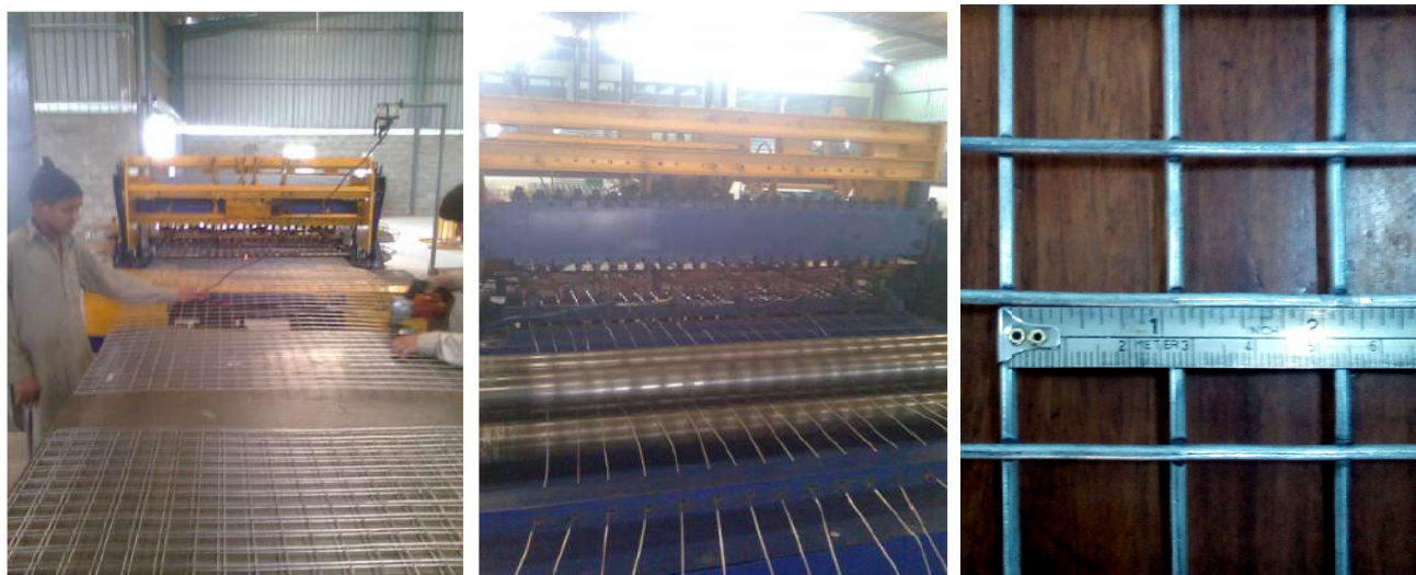
Figure 3. Preparation of spot-welded meshes.
