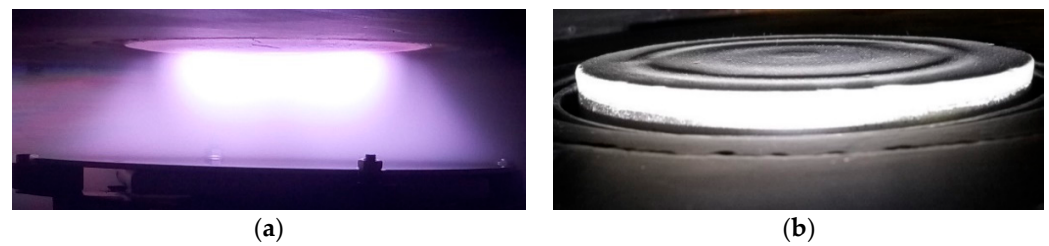
Figure 6. An RF magnetron discharge and a substrate holder (a), zone of HA target erosion after multiple deposition runs (b).
