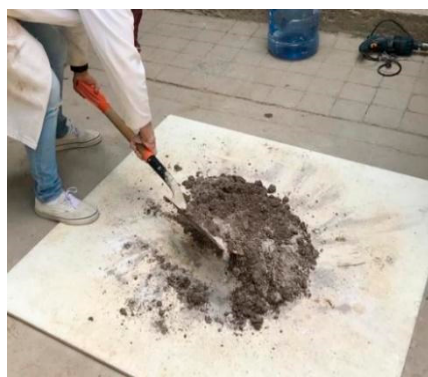
Figure 1. Mixing waste and cementing agents for Partition Block manufacturing.
