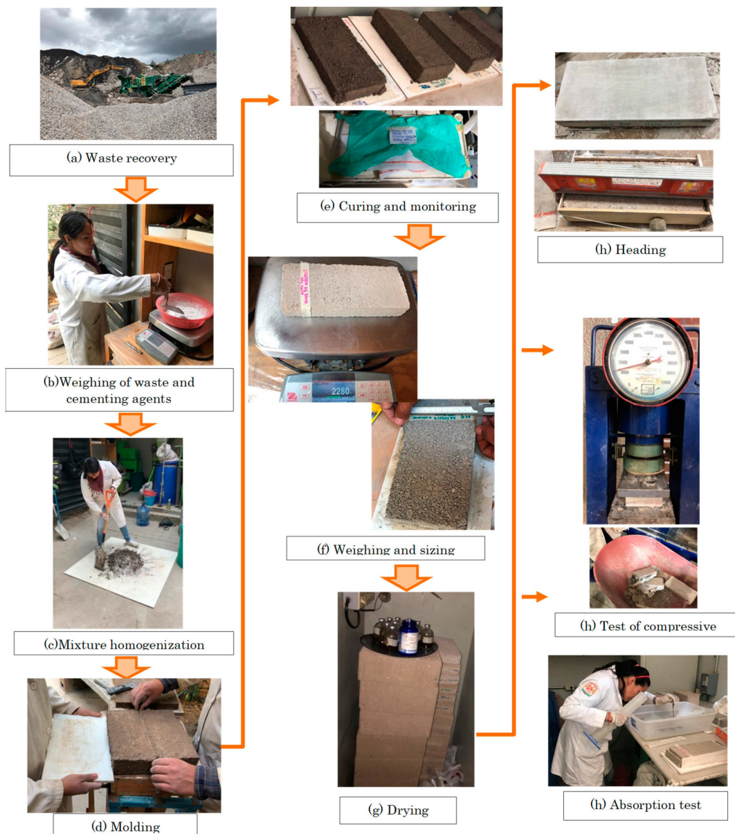
Figure 3. Specimen manufacturing process.
