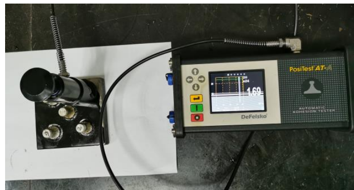
Figure 2. Portable automatic adhesion tester and testing configuration.
