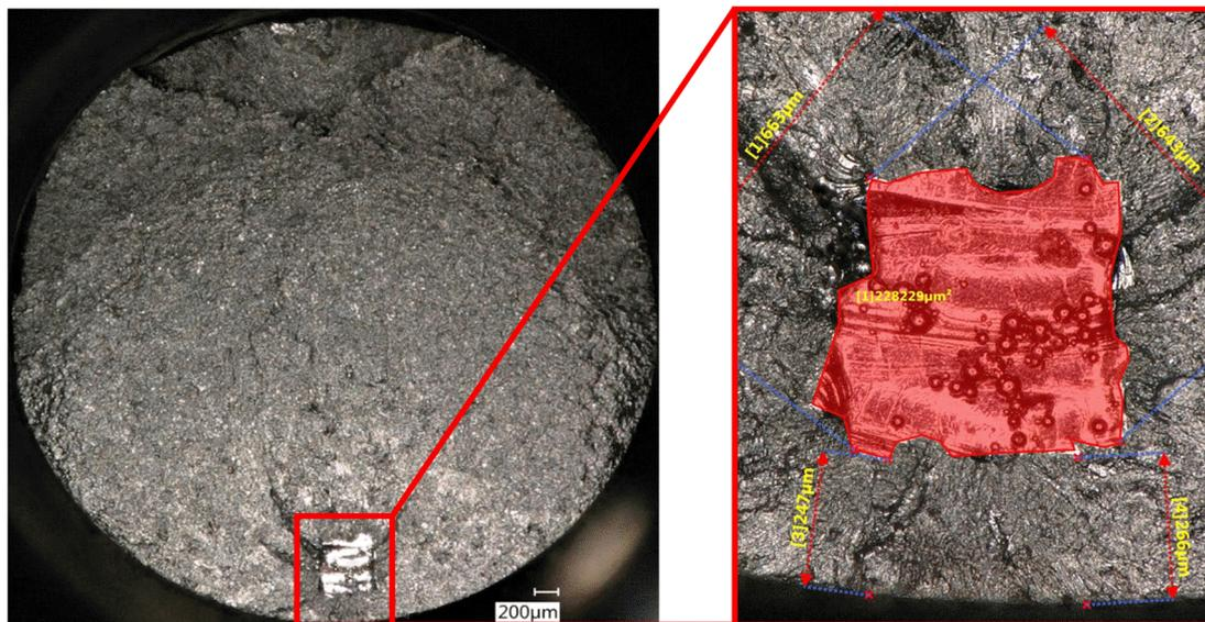
**Figure 12.** Defect area determination through fractographic analysis.
