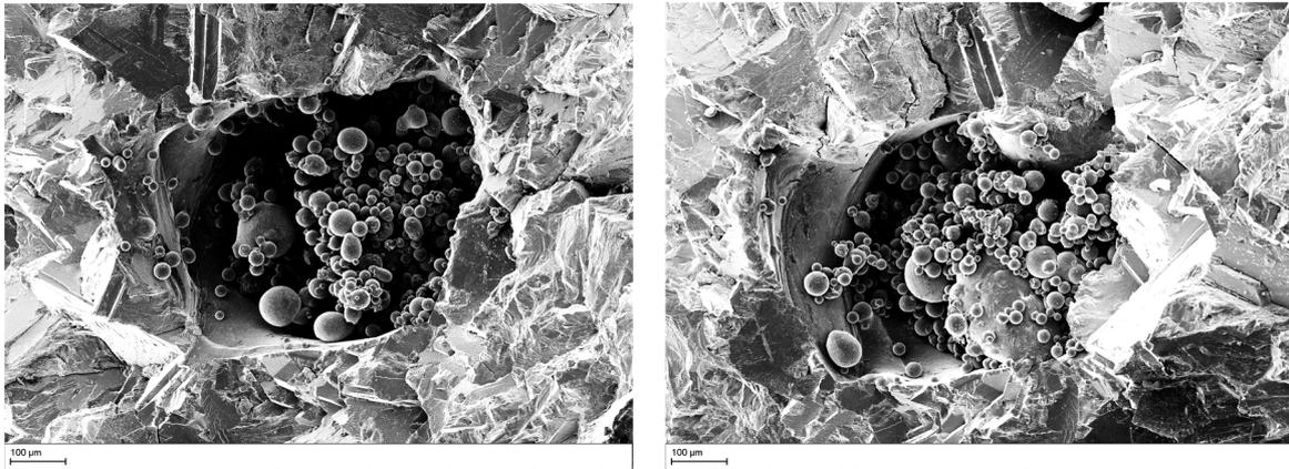
**Figure 7.** Typical failure location of Inconel 718 samples at the middle of the defect height. Top (**left**) and bottom (**right**) half on the same test coupon.
