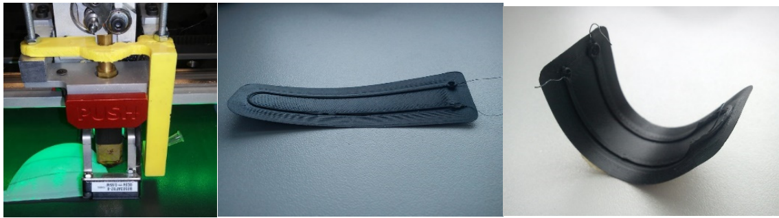
Figure 31. 3D printer head with additional nitinol applicator, samples of an actuator made by 3D printing.
