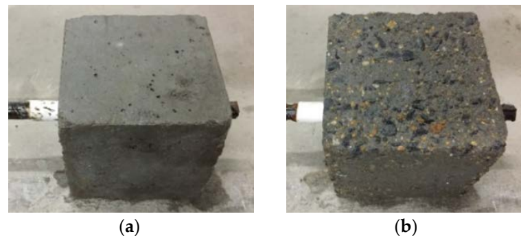
Figure 4. Appearances of concrete before and after freeze–thaw. (a) 0 cycle of salt frost; (b) 100 cycles of salt frost.
