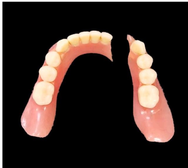
Figure 1. An example of a fractured acrylic denture base.
