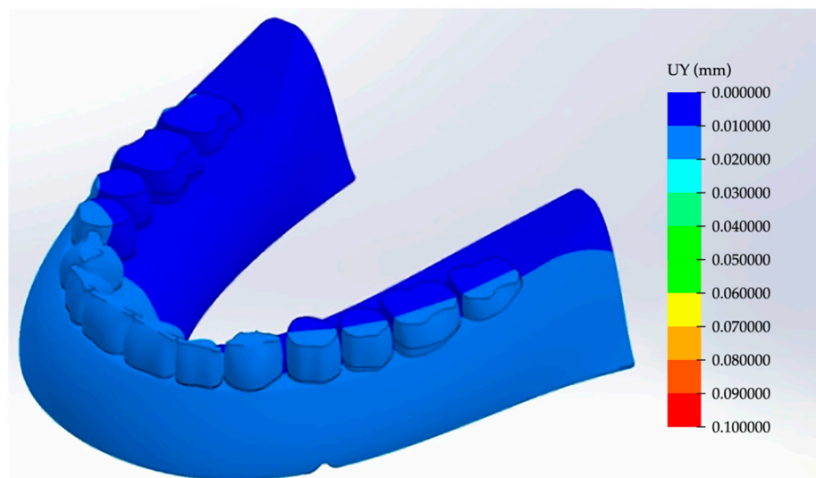
Figure 7. The schematic representation of the load distribution on the mandible RCDs base.
