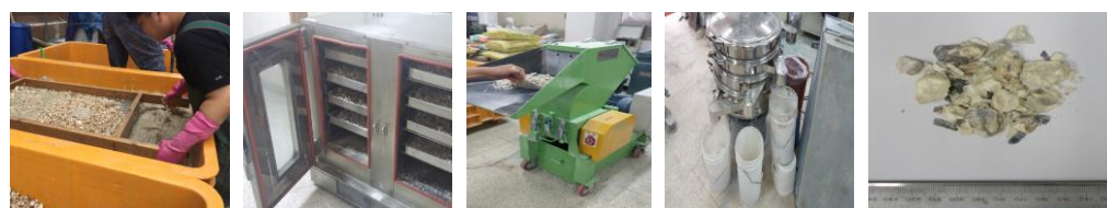
Figure 2. Conversion of oyster shells into OSA (washing, drying, grind in cutter mill, and classification in screen).
