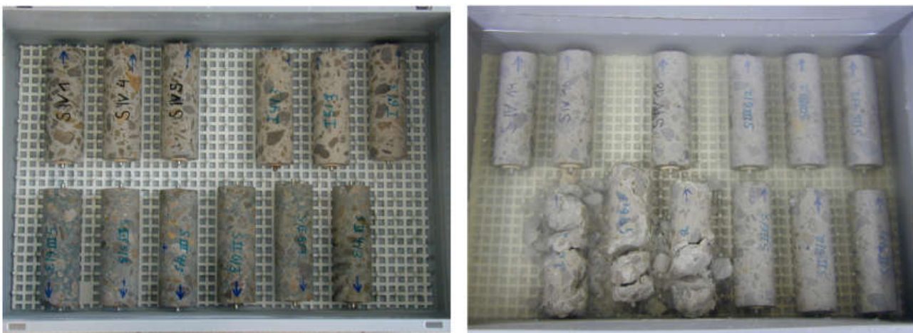
Figure 17. Concrete drill-out cores of type S I at the beginning of the test (left) and after 150 days of immersion in sodium sulfate solution (29.8 g/L) at 6 °C (right) [95].
