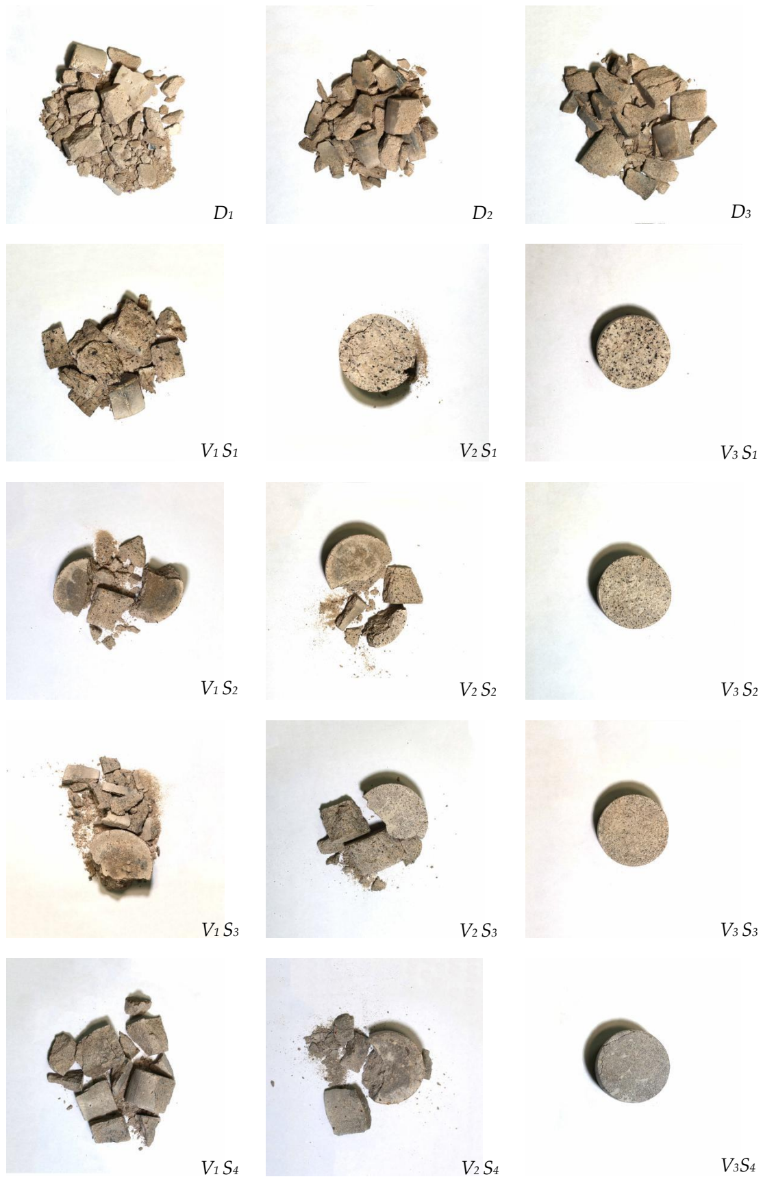
Figure 7. Fracture morphology of RASM specimen.
