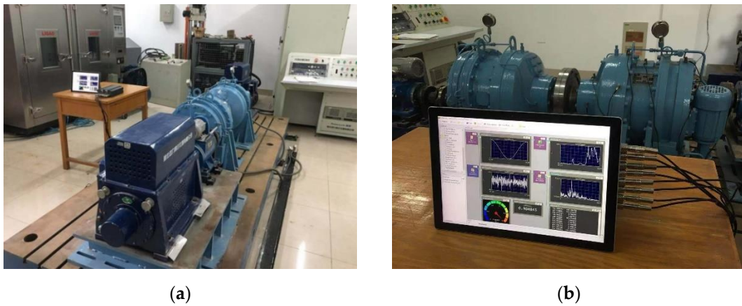
Figure 14. Bending fatigue test center. (a) Gearbox test bench. (b) Data acquisition and display.
