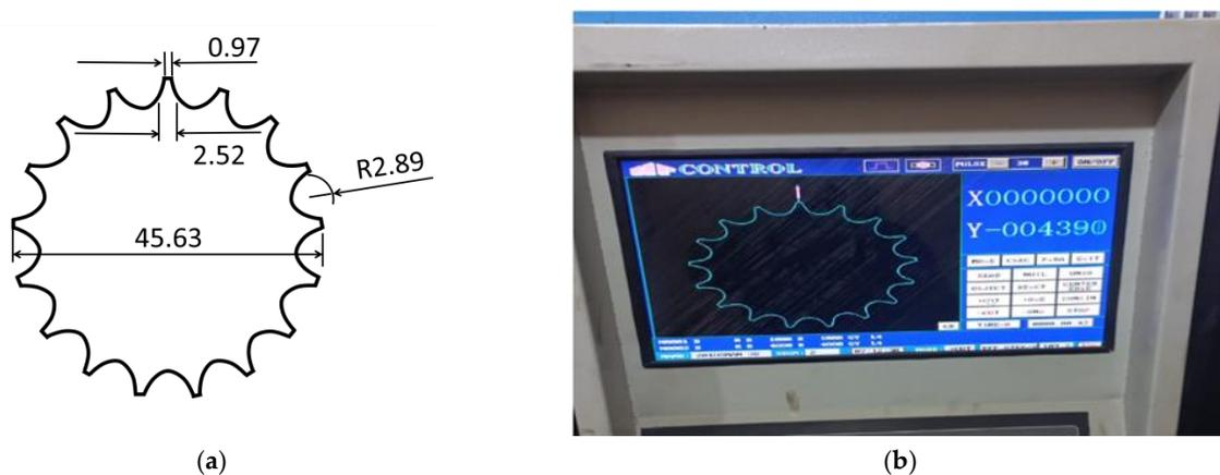
**Figure 4.** Wire cut electric discharge digital control machining showing (a) profile of timing chain sprocket gear teeth (all measurements in mm) and (b) the system working on a gear profile.
