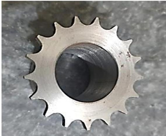
Figure 6. Final part design of timing chain sprocket.
