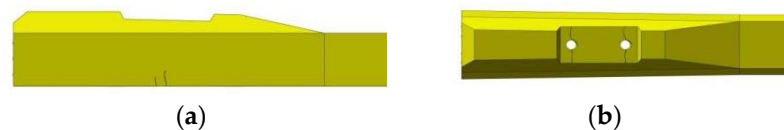
Figure 1. Transverse crack in a rail seat section: (a) lower part crack in the rail seat section; (b) upper part crack in the rail seat section.
