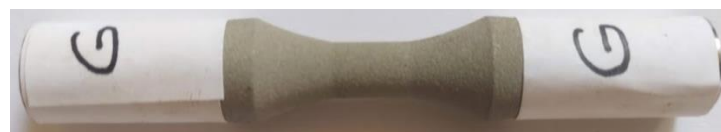
Figure 10. Sample G—unbroken after over 5 million cycles. \sigma = 318 MPa, n = 5,000,208 cycles.
