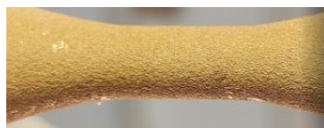
Figure 13. Macroscopic view of the surface of sample H (4340) after 5 million cycles.
