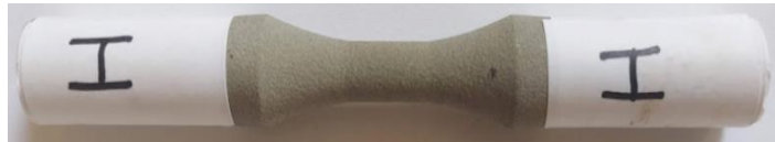
Figure 12. Sample H—unbroken after over 5 million cycles; \sigma = 346 MPa, n = 5,000,099 cycles.
