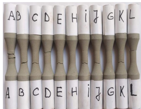
Figure 5. Samples after fatigue testing: A: static tensile sample; B–L: fatigue tested samples.
