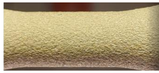
Figure 11. Macroscopic view of the surface of sample G (4340) after 5 million cycles.
