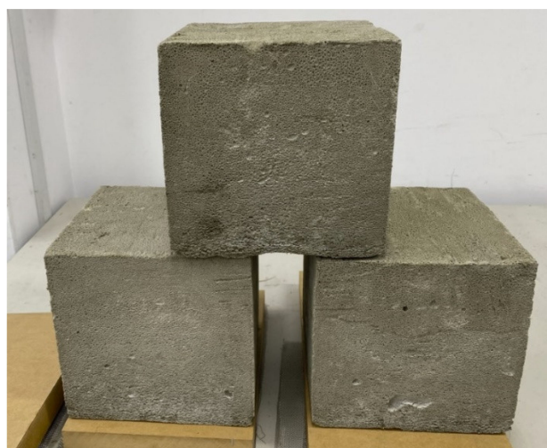
Figure 20. Three slab samples with a density of 0.2 \text{ g/cm}^3 .
