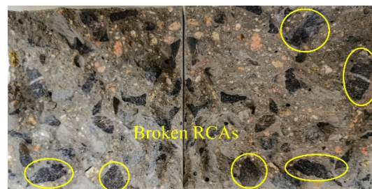
Figure 11. The typical destruction section of FRAC after splitting tensile destruction.
