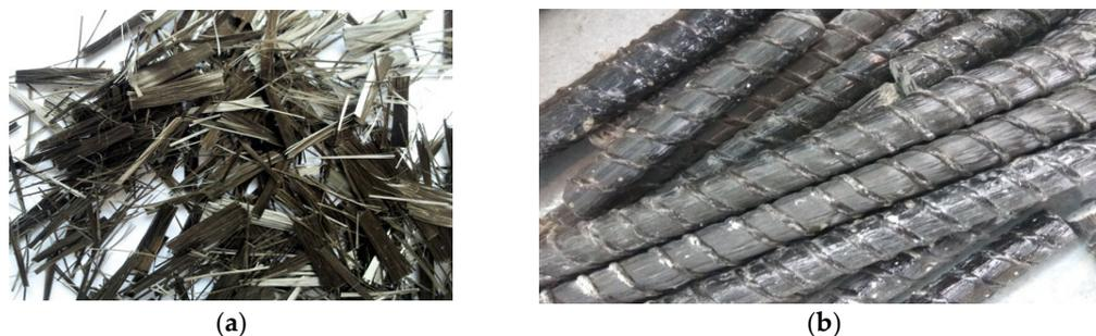
**Figure 1.** Reinforcement used in tests: (a) basalt fibers, (b) BFRP bars and stirrups.
