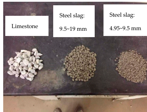
Figure 1. Aggregates of limestone and steel slag.
