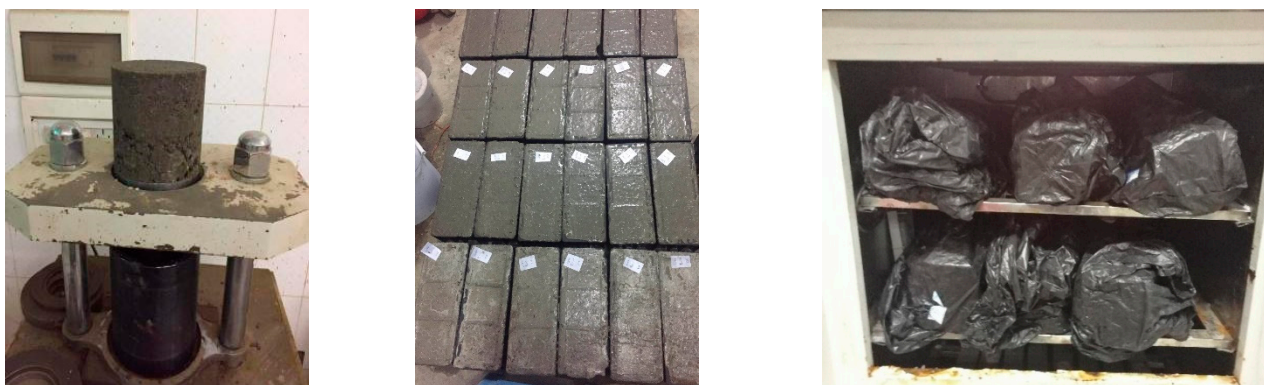
Figure 5. Specimen preparation and curing.
