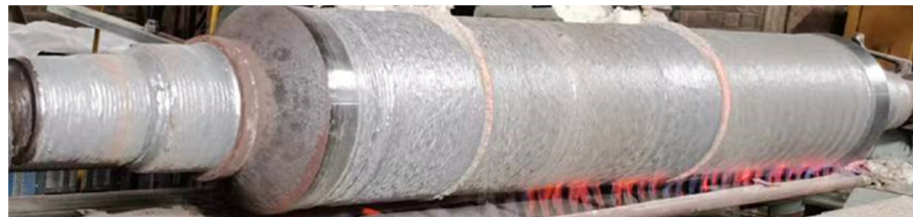
Figure 11. Roller repaired by the welding-hammering hybrid process.
