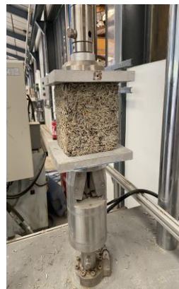
Figure 6. Compression strength test on rapeseed concrete.
