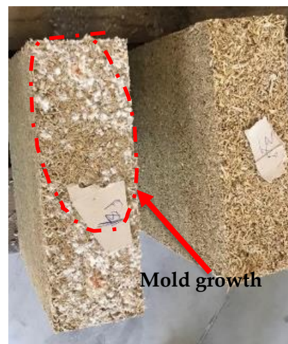
Figure 11. Rapeseed concrete samples made with the M-16 aggregates.
