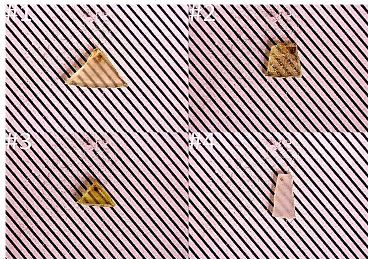
Figure 1. The samples under study: #1 LuAG:Ce SCF/YAG SC, h_{\text{SCF}} = 15 \mu\text{m} ; #2 LuAG:Ce SCF/YAG SC, h_{\text{SCF}} = 37 \mu\text{m} ; #3 LuAG:Ce SCF/YAG SC, h = 78 \mu\text{m} ; #4 YAG SC substrate (undoped).
