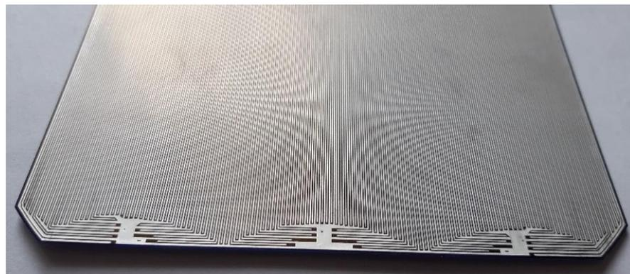
**Figure 7.** Rear surface of Maxeon Ne3 with visible connectors in the lower part.
