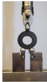
Figure 6. Experimental setups of O-ring multi-contact test for validation.
