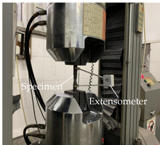
Figure 3. Tensile test setup.
