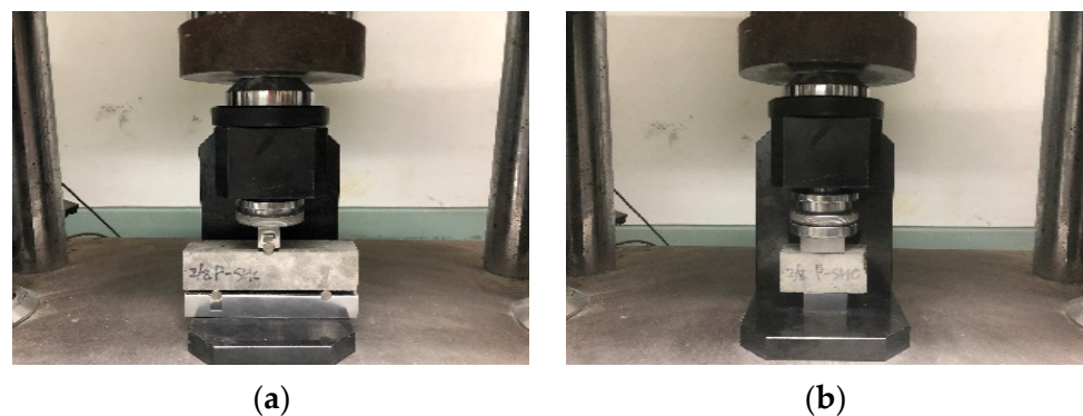
Figure 7. Experiment view: (a) flexural strength test; (b) compressive strength test.
