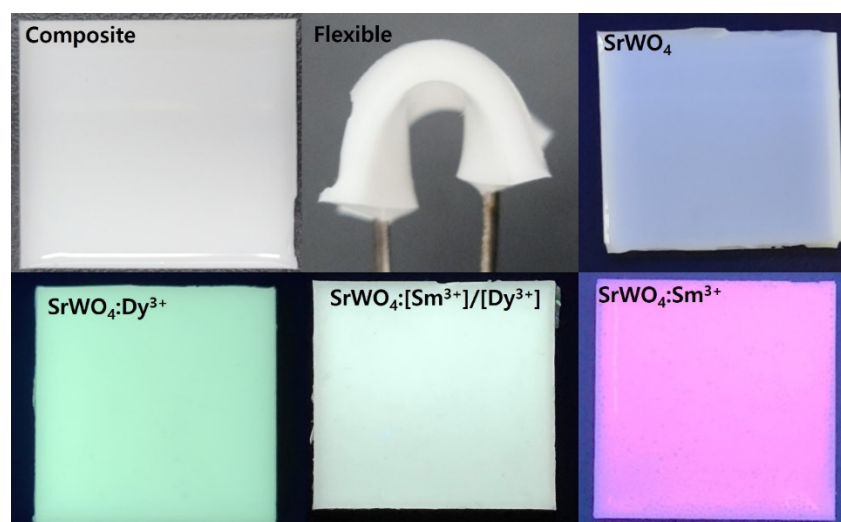
Figure 9. Images of flexible composite under daylight and UV light.
