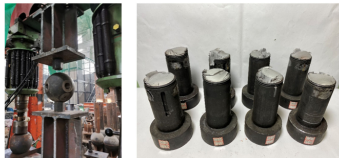
Figure 7. The M60 high-strength bolts that failed under fatigue loading.
