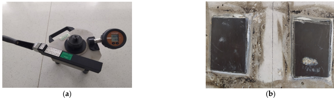
Figure 4. Pull-off testing device (a) and view of the CFRP tape pieces glued to the cleaned surface (b).
