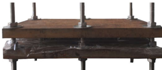
Figure 3. The fixture utilized for the fabrication of SLJs and AFSs.
