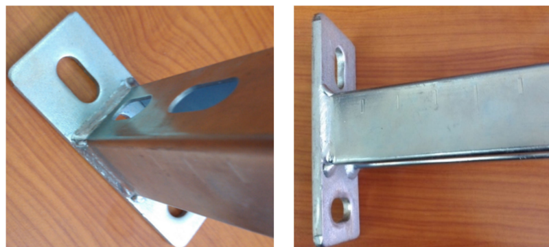
Figure 2. Example of a welded console—a close look at the weld zone after regalvanizing; standard profile of 40 mm × 40 mm cross-section dimensions.
