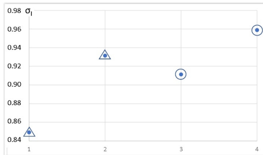
Figure 17. The calculated indicator \sigma_1 for consoles with selected locks: 1—arrow lock; 2—arrow lock with dash; 3—semicircular lock; 4—semicircular lock with dash.
