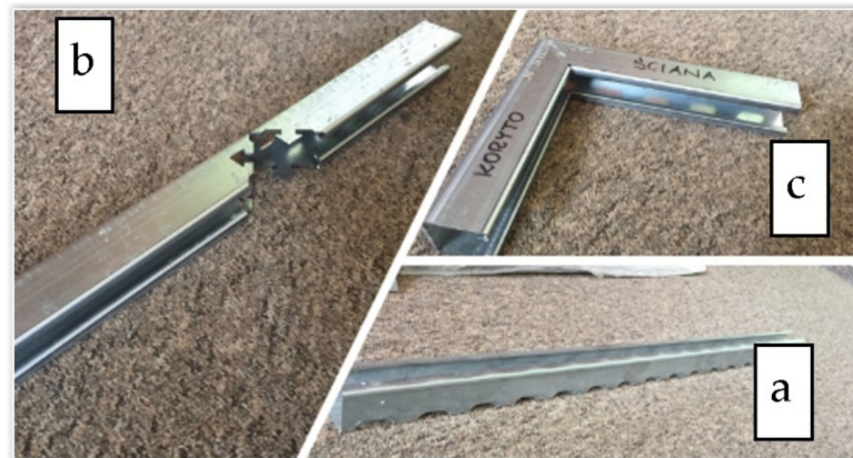
Figure 4. The profile section obtained on the roll-forming line (a); a profile section after a laser cutting of a zipper/lock (b); and a console with a lock after assembling (c). Standard profile of 40 \times 40 mm cross-section dimensions.
