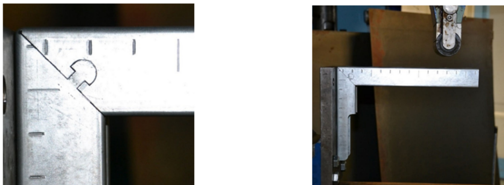
Figure 20. Correctly made console with a semicircular lock in close-up; console before loading on the experimental stand (40 mm × 40 mm profile).
