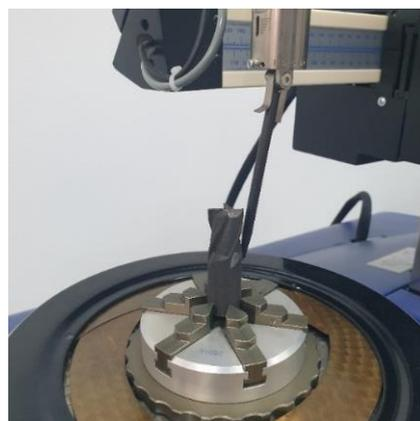
**Figure 5.** Measurement of the roundness and cylindricity profiles of the shank.
