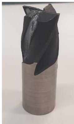
**Figure 6.** General view of the 3D printed tool.
