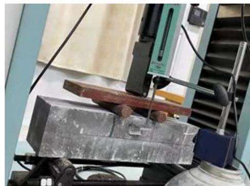
**Figure 4.** Device of flexural strength testing.
