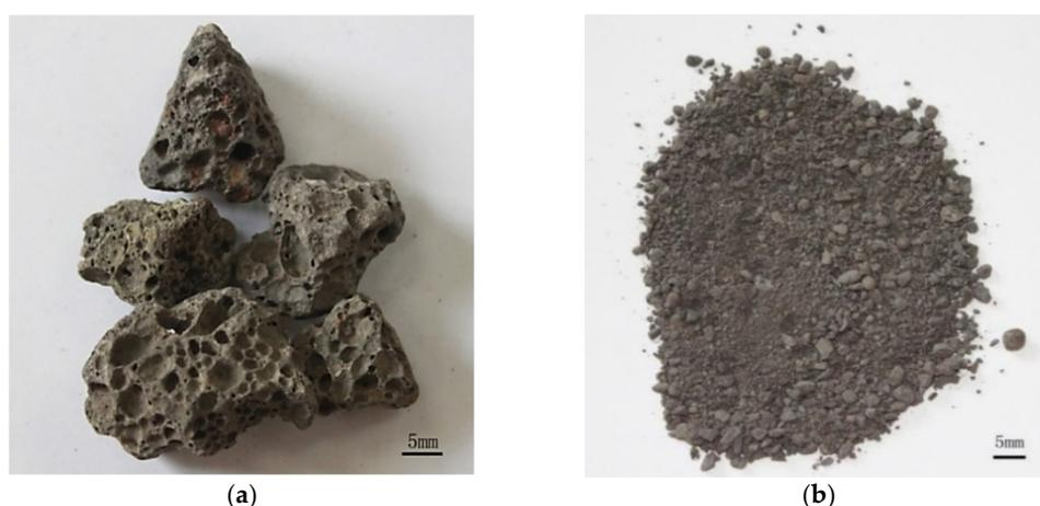
**Figure 1.** Appearance of high titanium heavy slag. (a) coarse aggregate, (b) fine aggregate.
