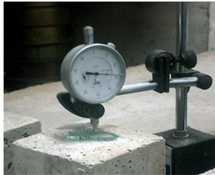
**Figure 5.** Drying shrinkage testing of concrete.
