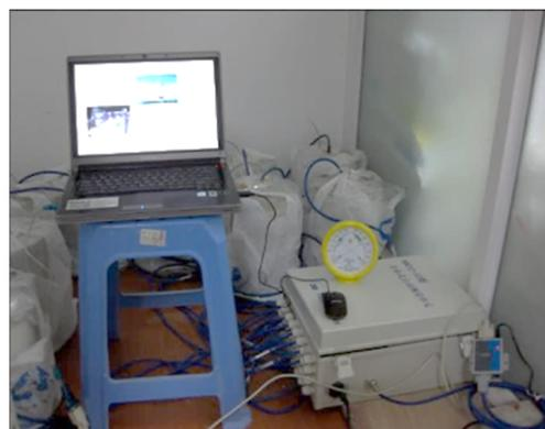
**Figure 7.** Autogenous shrinkage and internal humidity testing.
