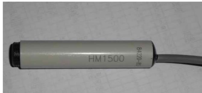
**Figure 6.** Moisture meter embedded in concrete.
