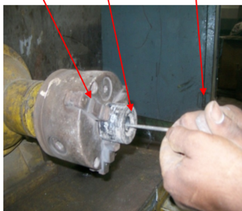
Figure 2. Hand polishing of die by the skilled operator.
