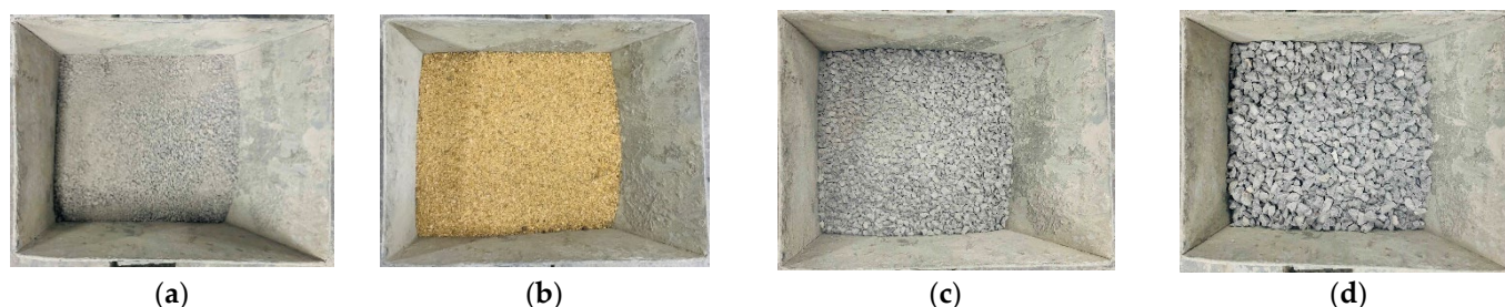
Figure 3. Pictures of aggregates: (a) manufactured sand; (b) river sand; (c) 5~10 mm aggregate; (d) 10~16 mm aggregate.
