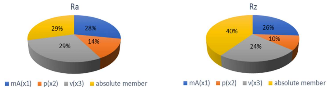
Figure 12. Graph of significance of mathematical model parameters for Ra and Rz roughness parameters.
