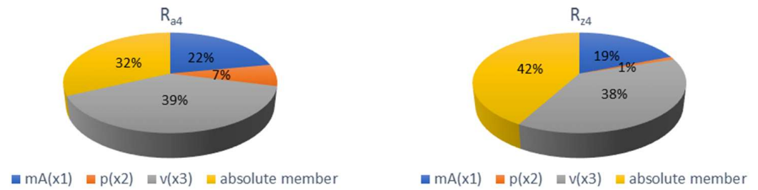
Figure 13. Graph of significance of mathematical model parameters for Ra_4 and Rz_4 roughness parameters.
