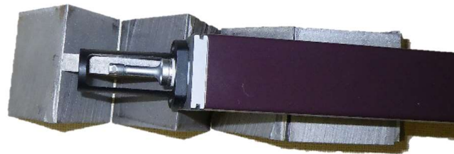
Figure 5. SurfTest SJ-301 device measuring the roughness of the cut surface.
