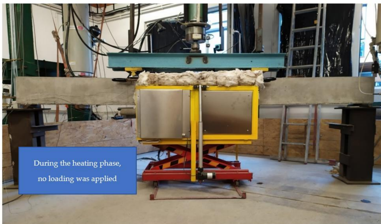
Figure 3. Test setup during the heating phase (set 1.1—sample B2Ø14).
