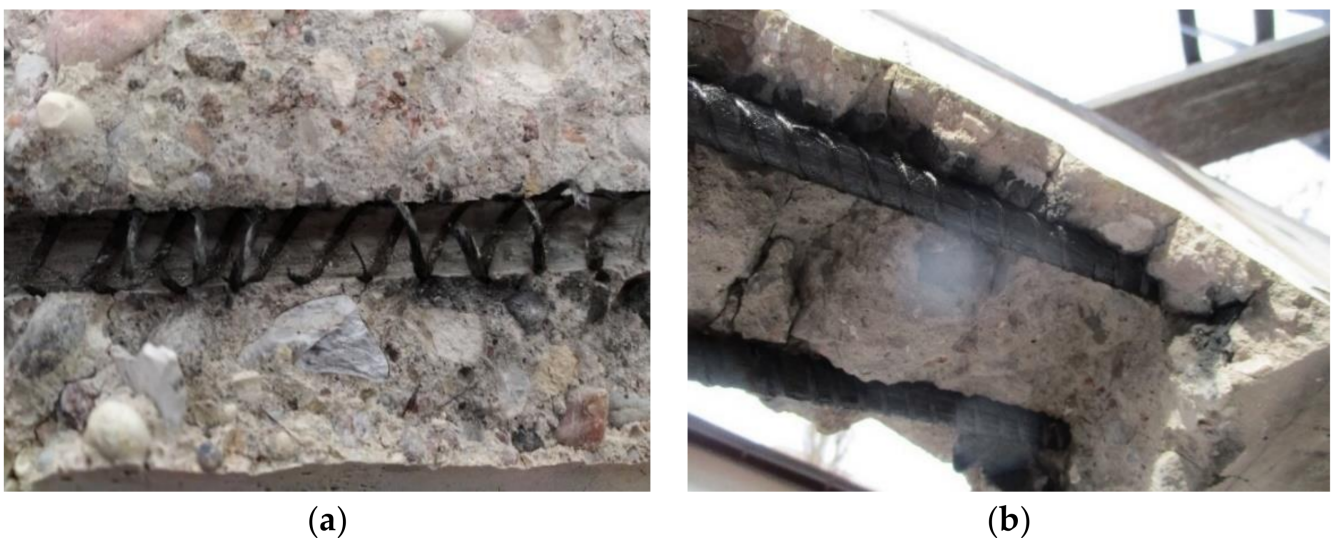
Figure 7. Removal of bars from concrete beams: (a) middle part of the beam; (b) side part of the beam.
