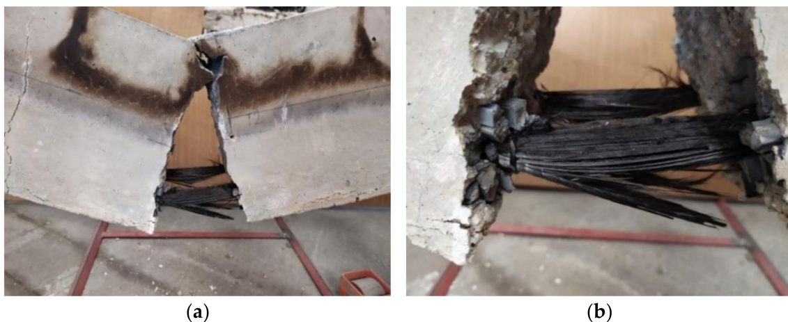
Figure 5. Destruction of specimen B2Ø14: (a) non-magnified image; (b) magnified image.
