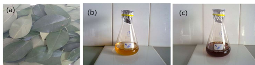
Figure 1. (a) L. Lucidum plant leaves; (b) Leaf extract and aqueous solution of \text{AgNO}_3 ; (c) synthesis of silver nanoparticles.
