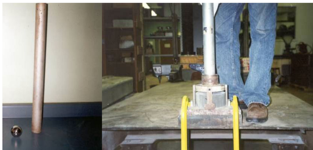
Figure 5. Impact test apparatus and testing of mortar composite using cylinder specimen.
