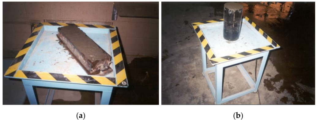
Figure 3. Beam (a) and cylinder (b) specimens cast for flexure and impact tests.
