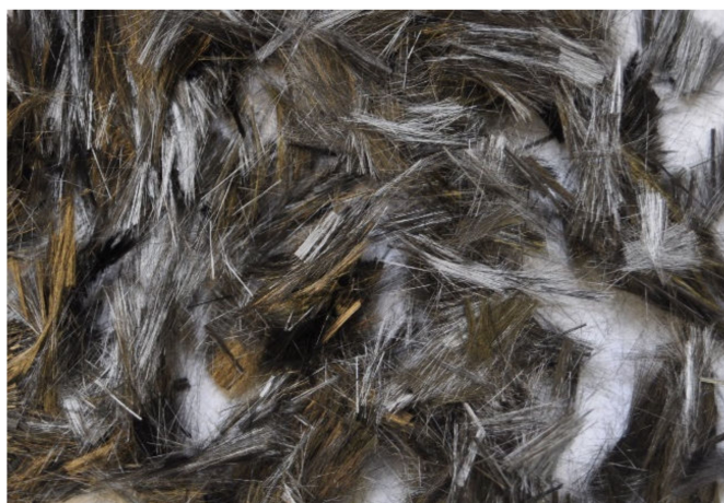
Figure 1. Short pitch-based carbon fibers used in various mortar composites.
