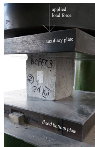
Figure 5. Experimental test of the compressive strength.
