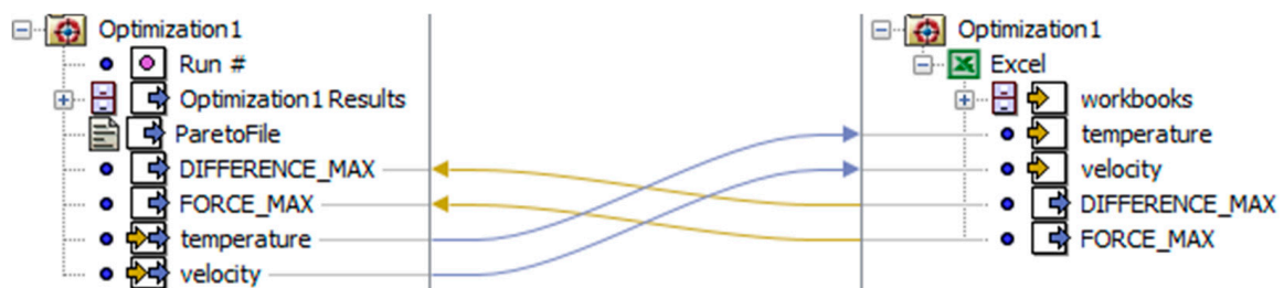
Figure 23. Exemplary view of the connection between particular parameters during optimization using MS Excel and Simulia Isight software.
