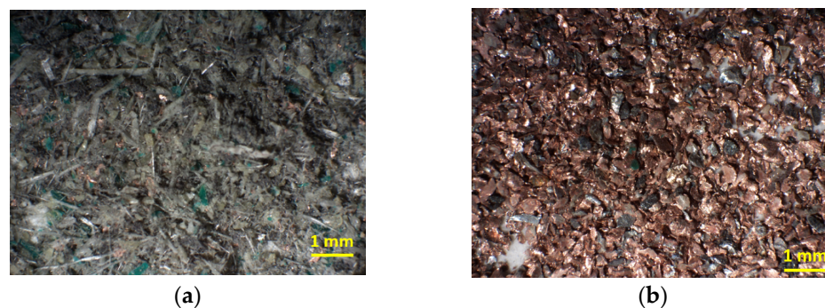
Figure 4. Nonconductive (a) and conductive (b) products resulting from electrostatic separation for the class size <0.3 mm.
