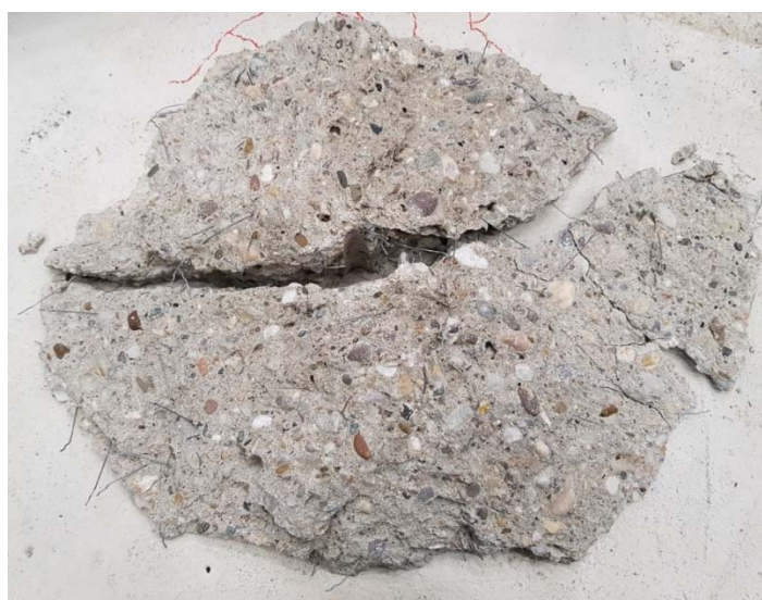
Figure 6. Representative concrete cone breakout body (bottom view).
