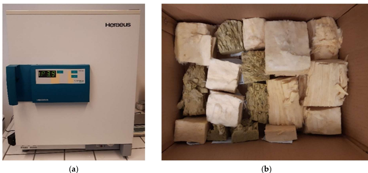
Figure 6. (a) Dryer Heraeus Function Line UT6P; (b) Samples after reaching a stable weight.
