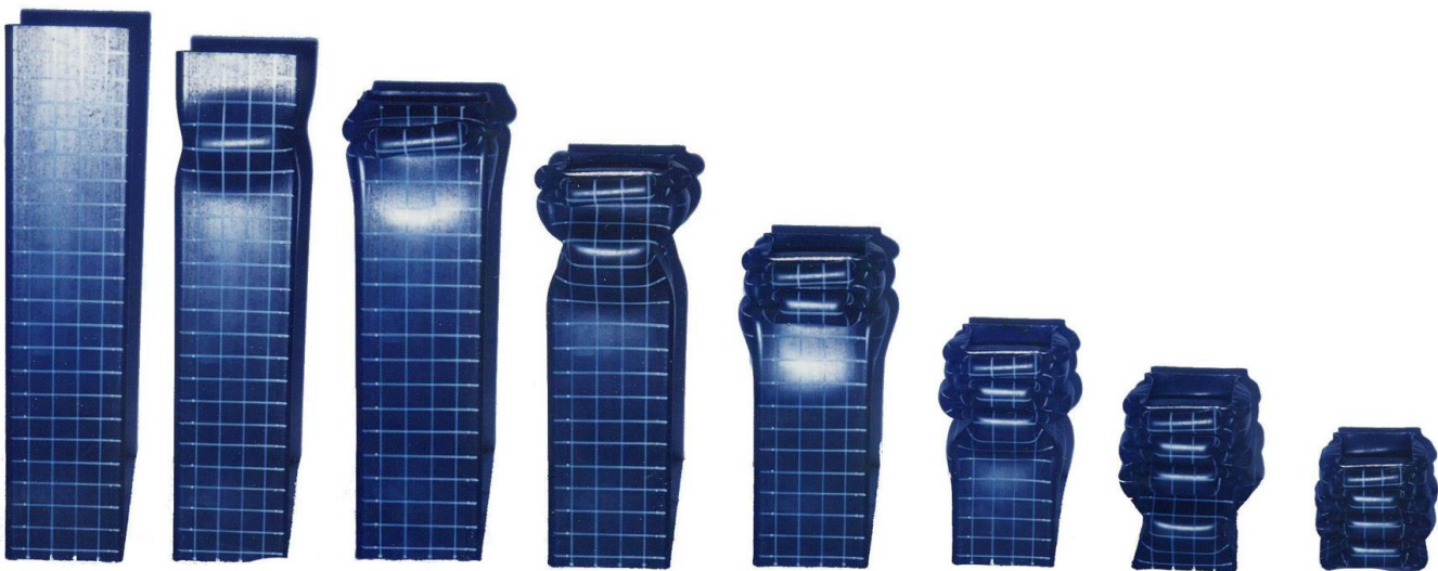
Figure 4. Crushing test of an unstiffened specimen in the experimental work (US-1).
