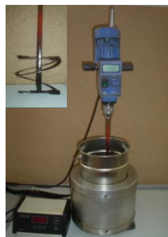
Figure S2. Apparatus to produce asphalt rubber at the laboratory.
