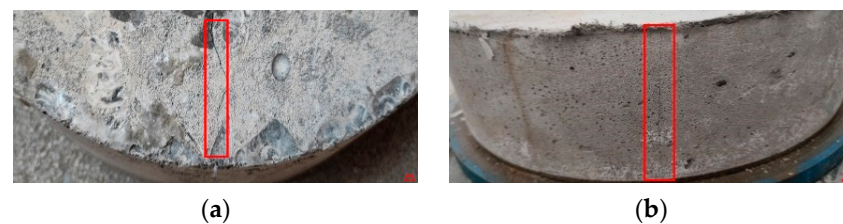
Figure 18. Crack status. (a) Concrete; (b) SSPP-ECC.
